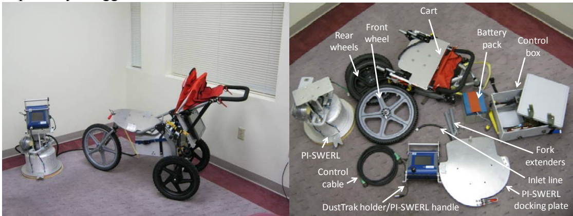
Figure 2-1 Miniature PI-SWERL Measurement System. Left - fully assembled, right - principal components.
